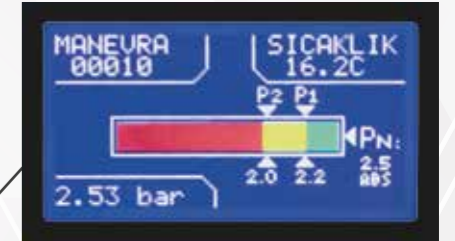
Possibility of SF6 gas pressure and temperature control from large screen digital manometer with double contact and possibility of tracking the number of maneuvering of the disconnecter.
