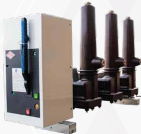
Circuit breaker with SF6 gas is used which has the class of M2 E2 C2 (10.000 mechanical operations). Vacuum circuit breaker is also used optionally.
