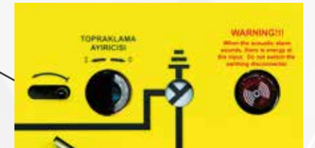
Operator-friendly illuminated and audible warning system that warns in the movement of the operator in the earthing switch when there is energy at the entrance and warns to avoid closing the earthing switch on energy.
